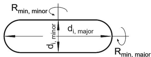
**Inner dimensions,  $d_i$ , of flat duct and minimum radius of curvature,  $R_{\text{min}}$ ,
