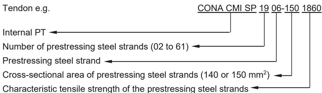
The tendons comprise 01 to 61 tensile elements, 7-wire prestressing steel strands according to Annex 30.
